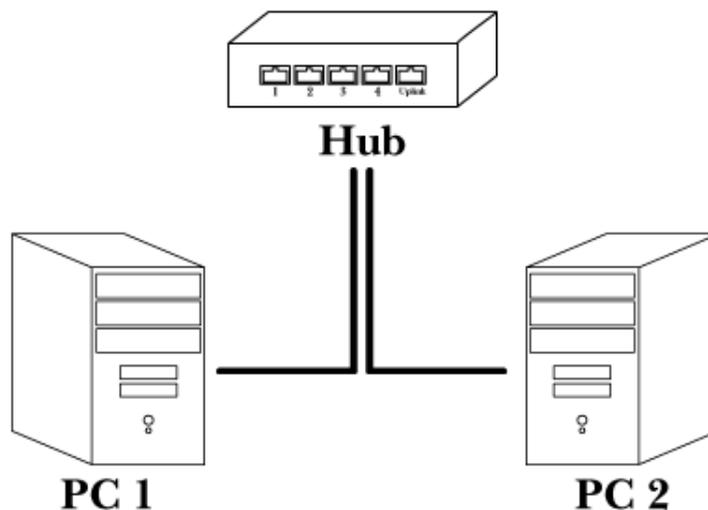
In the figure above, two ordinary computers have a network card installed in them, and a network cable connecting each of them to a network hub or switch. In a simple network, that's really all there is to it. But, like most things in life, there's more than meets the eye.
